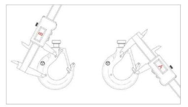
PROLH lever hoists are fitted with the patented Tiger "EZ check" 3 point marking system. With this system a quick check that the A and B measurements are the same (as shown in the diagram below) will indicate if the hooks have stretched If  $A \leq B$  the hook is fine; If A > B the hook needs to be replaced.
