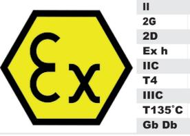
**Equipment Group: surface inc** Category: High Safety - Ex At **Category: High Safety - Ex At Protection type: Design safet Gas Explosion Group: Protect Gas Temperature Class: Max Groups of Dust: Protected for Dust Temperature Class: Max Equipment Protection Level**
