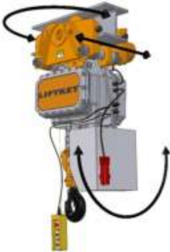
Diagram No. 15: Freedom of movement between the hoist and the trolley
