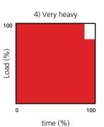
Hoists which regularly lift loads approximately equal to the maximum load.
