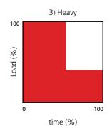
Hoists which frequently lift the maximum load but normally medium loads.
