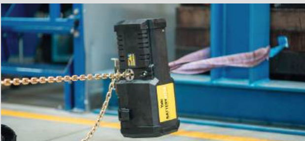
Horizontal pulling by remote control, also in places without power supply.
