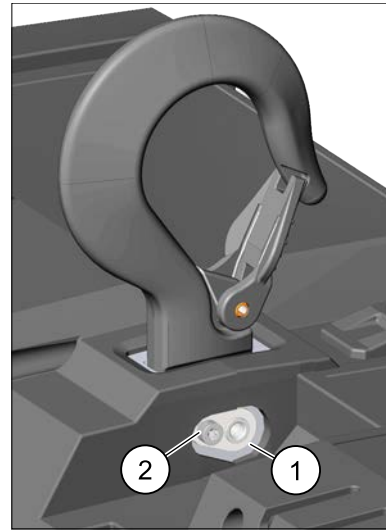
Figure 7. Suspension Pin Retainer/Retainer Screw
